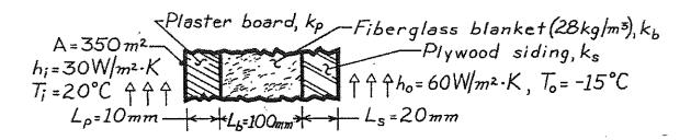
**PROPERTIES:** Table A-3,  $(\overline{T} = (T_i + T_o)/2 = (20-15)^\circ \text{C}/2 = 2.5^\circ \text{C} \approx 300\text{K})$ : Fiberglass blanket, 28 kg/m<sup>3</sup>, k<sub>b</sub> = 0.038 W/m·K; Plywood siding, k<sub>s</sub> = 0.12 W/m·K; Plasterboard, k<sub>p</sub> = 0.17 W/m·K.
