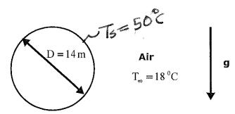
The density of air at 1500 m is  $\rho$  = 1.059 kg/m³. The remaining air properties do not change with altitude.
