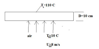
Determine the rate of heat loss from the pipe per unit of its length.
