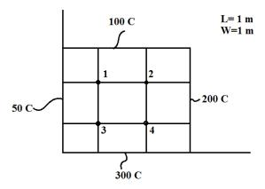
a) Determine the temperatures at nodes 1,2,3 and 4. Estimate the midpoint temperature.
