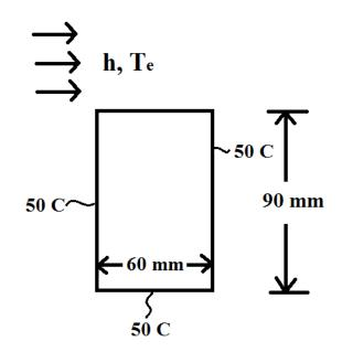
Using a grid spacing of 30 mm determine nodal temperatures and heat rate unit length normal to the page into bar from the air.
