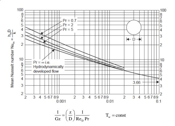
Equations (a) and (e) can be used in conjunction with the appropriate correlation for the Nusselt number, and the two unknowns L/D and  $\overline{Nu}_D$  can be found.
